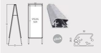
The Poznan A-board frame is made of aluminum so it is lightweight and resistant to rusting and it is available on black or silver color. It has a 32mm width profile with click system, so the graphic change is quick and simple. It includes a weather resistant antireflection protector which allows it to be read under bright lights. Thanks its double-sided frame and its 1800mm height this A-Board is ideal for advertising large offers, menus, information maps, etc, outside or inside your business.
