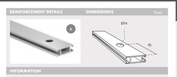
When the TexFix® exceeds 2monone of its sides, it is necessary to use the Central Reinforcement to ensure the stability of its structure. Made of aluminum and its assembly is very simple, you just have to make two holes of 14mm diameter at a distance of 45mm at its ends. In this way, the Locks are introduced at both ends and next to the reinforcement they are connected to the TexFix® profiles.
