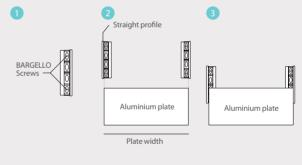
Possibility of fixing with double sided tape. Continue with the next steps if you wish to screw it to the wall:
