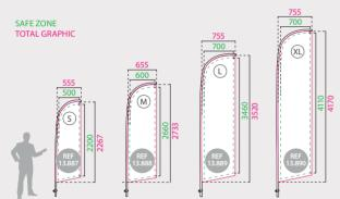
The Knife is a flagpole made of fiberglass, aluminium and plastic. The pole is collapsible for an easy portability. Also, a nylon carry bag is included. Multiple accessories are available later at this chapter. Textile manufacturing is available (not included). You can choose A white or **B**black colour of pole sheath.
