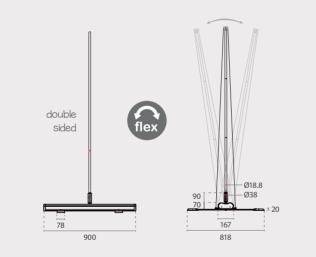
Ibiza RollUp features a silver aluminium finish and it is suitable for outdoor or indoor use. Its design features a flex system for resisting wind. Feet are holed for being used with 4 stakes (included). It is ideal for areas with 2-ways traffic.
