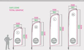
The Knife is a flagpole made of fiberglass, aluminium and plastic. The pole is collapsible for an easy portability. Also, a carry nylon bag is included. Multiple accessories are available later at this chapter. Textile manufacturing available (not included). You can choose A white or **B** black colour of pole sheath.
