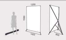
Valoria X-Banner is a portable, detachable and lightweight display for interchangeable graphics. Its X-shaped structure is made of fiberglass and plastic parts. Exhibitors can quickly assemble it in a few seconds (no tools required). It includes a nylon carry bag. Because of its 1200mm width they are suitable for joining multiple units as a photocall or a promotional wall.
