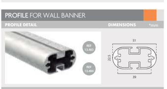
Lightweight profile made of anodised aluminium, available in 2 or 3m length.
